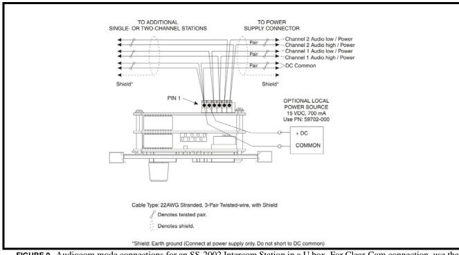
**FIGURE 9.** Audiocom mode connections for an SS-2002 Intercom Station in a U box. For Clear-Com connection, use the *Unbalanced Mode Intercom Channel* pin out information listed in "Specifications" on page 18.
